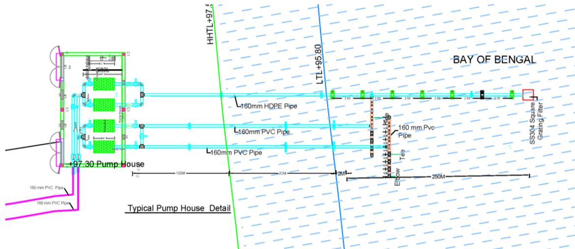
1. **Sea Water Intake System:** Two types of intake suction line have been installed in the project as below
